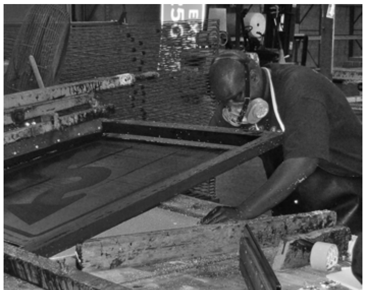
Lee Greene uses a silk screen to apply an arrow onto reflective sheeting.
