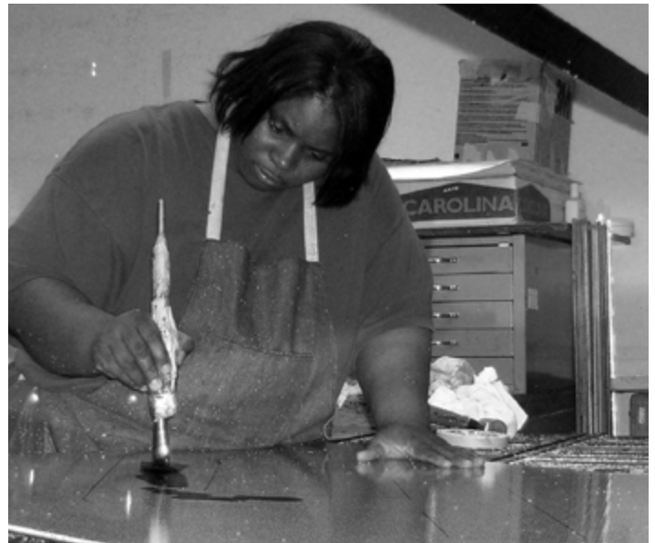
AHTD Sign Layout Specialist Marilyn Embry hand paints an arrow onto a road sign.
