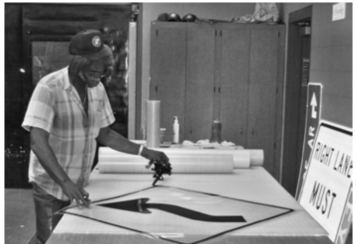
Gene Morrison applies a stencil onto a sign and prepares it for delivery.
